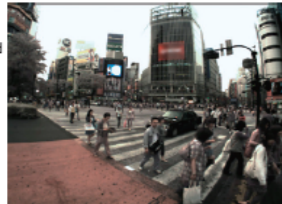
Standard wide angle lens f=3.3mm (horizontal angle 104.3°)
